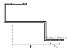
**Fastening to the substructure: (acc. to DIN 1052)**     $e_D = 50 \text{ mm}$      $e_S = 50 \text{ mm}$
