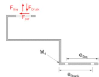
**Fastening to the substructure: (acc. to DIN 1052)**     $e_D = 50 \text{ mm}$      $e_S = 50 \text{ mm}$
