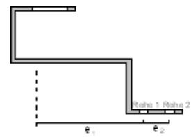
**Fastening to the substructure: (acc. to DIN 1052)**     $e_D = 50 \text{ mm}$      $e_S = 50 \text{ mm}$
